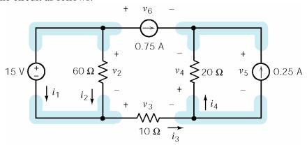
The subscripts suggest a numbering of the circuit elements. Apply KCL at node b to get
