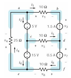
Apply Ohm's law to each of the  $10 \Omega$  resistors to get
